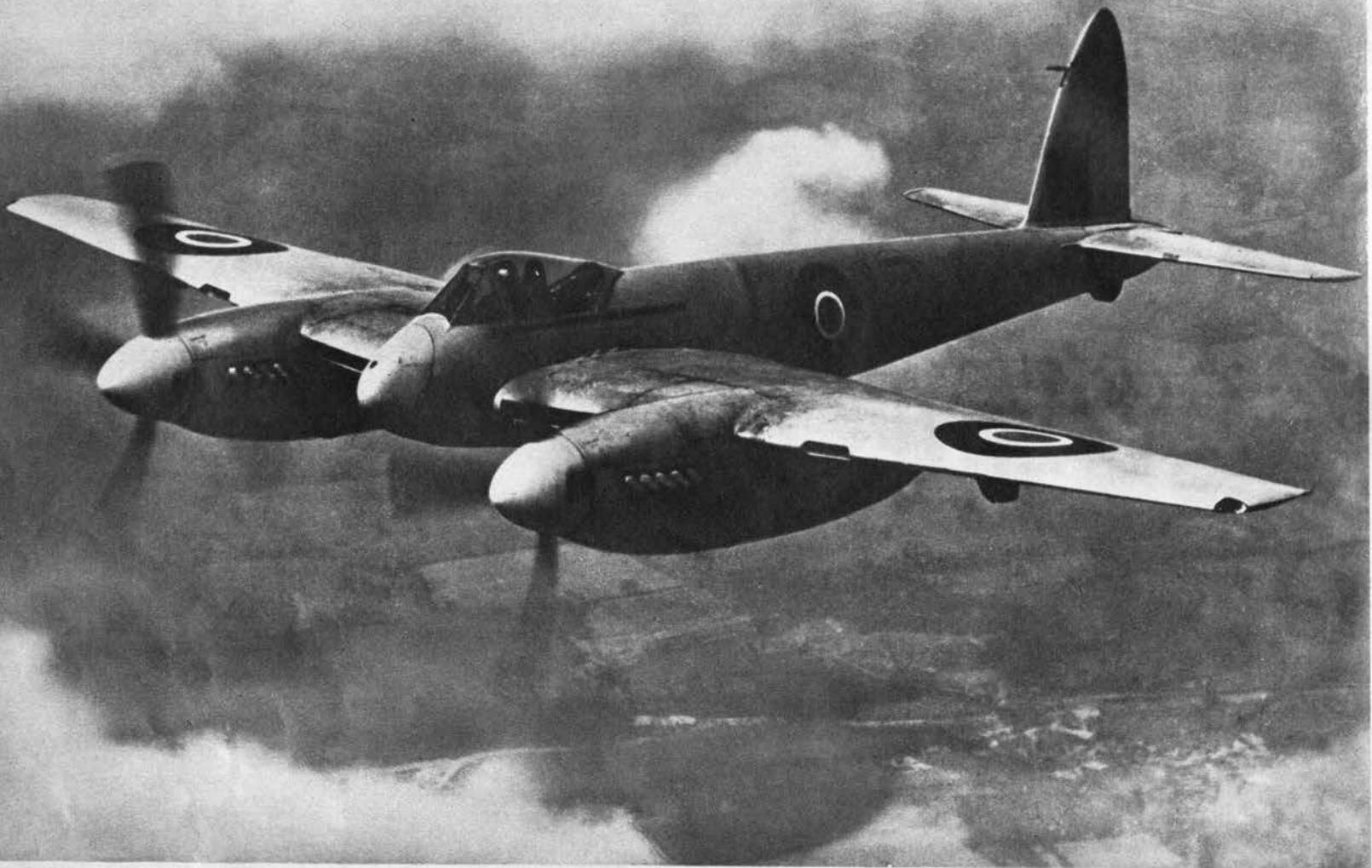
SINGLE-SEAT HORNET LOOKS LIKE SLIMMER MOSQUITO. TOP SPEED OF ABOUT 470 M. P. H. MAKES IT ONE OF FASTEST PROPELLER-DRIVEN PLANES
